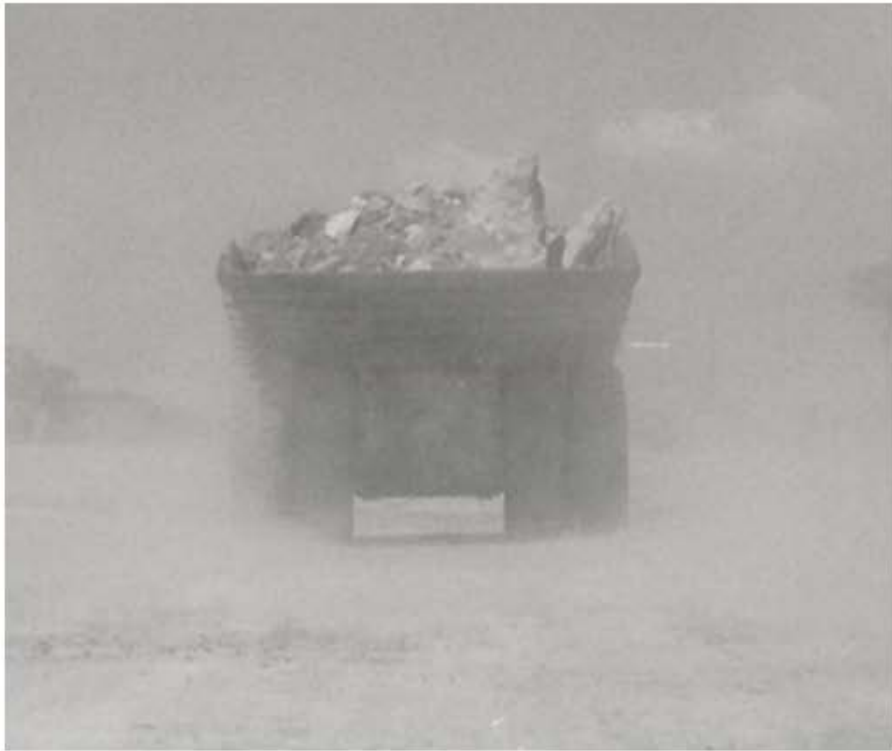
Untreated Road Section Heavy Dusting
