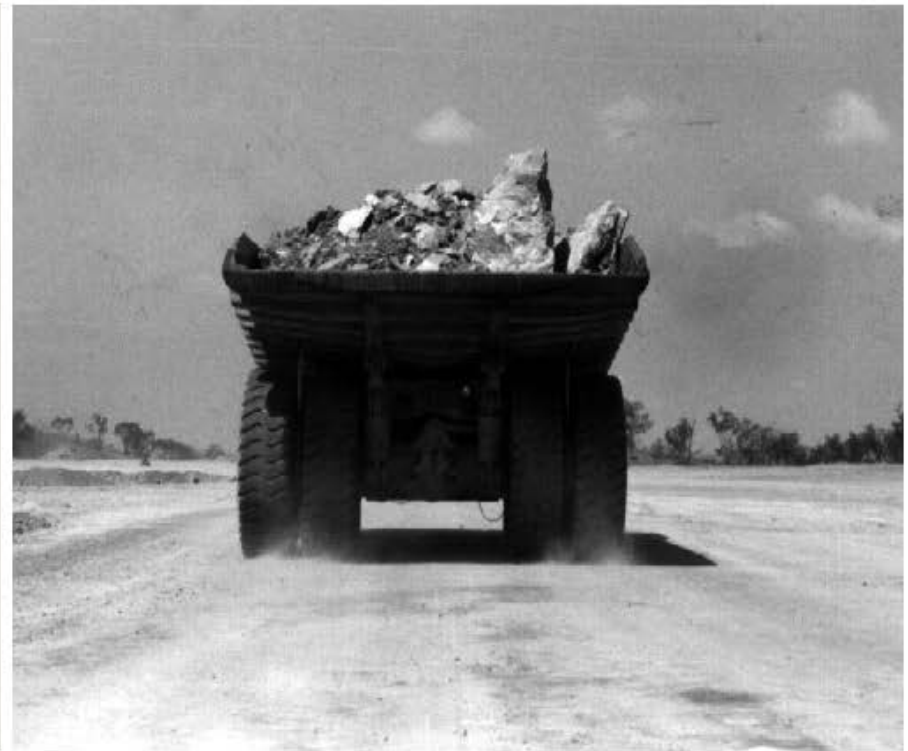
Same Truck on Treated Surface Minimal Dusting
